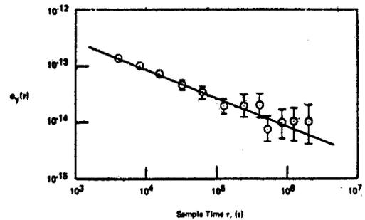
Fig. 5. Frequency stability of two high performance commercial caesium beam standards.
