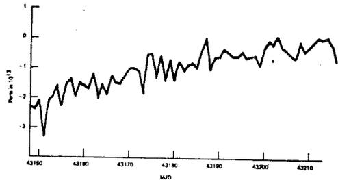
Fig. 2 Frequency vs. time of commercial caesium.
