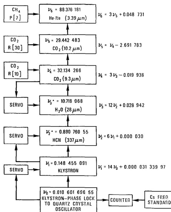
Fig. 2. Stabilized infrared frequency synthesis chain. All frequencies are given in terahertz. Wavelengths are stated in parentheses.
