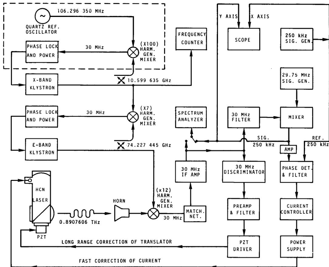
Fig. 5. Laser stabilization scheme.
