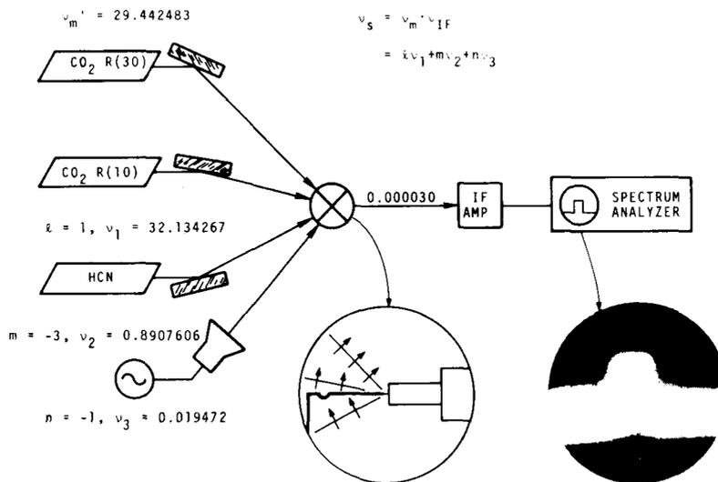
Fig. 1. Example of infrared frequency synthesis with HCN laser. All frequencies are given in terahertz.
