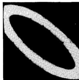
Fig. 7. 250-kHz Lissajous figure where Y axis is driven by down converted beat note and X axis is driven by phase-detector reference.
