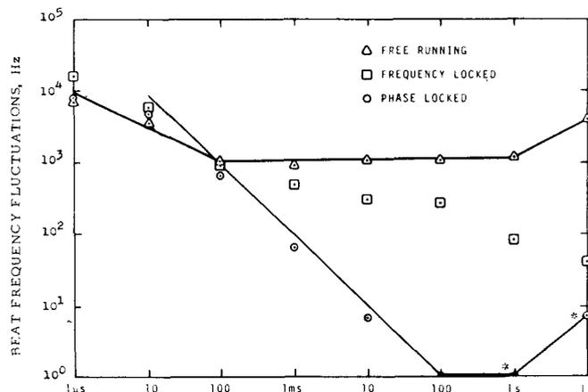
Fig. 8. HCN laser stability as measured with computing counter. Vertical scale is square root of Allan variance,  $\sigma_{\delta\nu}^2(N, T, \tau, B)$  of the frequency fluctuations for  $N = 2$ ,  $T - \tau \approx 3$  ms, and  $B = 200$  kHz.
