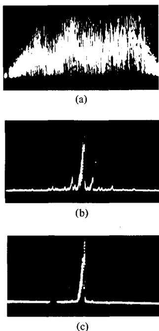
Fig. 6. Beat notes between laser and microwave reference chain, down converted to 250 kHz. Vertical scale is linear, dispersion is 200 Hz/division, resolution is 20 Hz, and sweep rate is 5 s/div. (a) Laser is frequency locked. (b) Laser is phase locked. (c) For comparison with (b), the spectrum of 250-kHz reference to phase detector is shown. Dispersion, resolution, and sweep time are unchanged.
