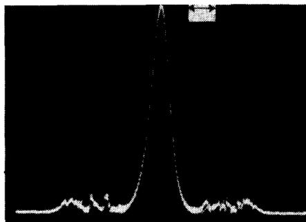
Fig. 9. Phase-locked beat note at 30 MHz. Vertical scale is linear, dispersion is 20 Hz/div, bandwidth is 10 Hz, and sweep rate is 2 s/div.
