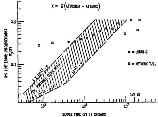
Fig. 10. Estimation of the rms time dispersion versus sample time for Loran-C, 3-network TV line-10, and cesium portable clock techniques with USNO and NBS as the time references
