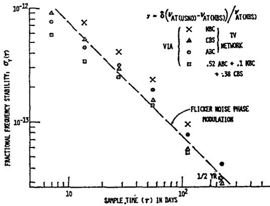
Fig. 4. Fractional frequency stability,  $\sigma_y(\tau)$ , of the AT(USNO) — AT(NBS) time scales compared by the 3-network TV line-10 technique
