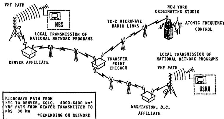
Fig. 1. Typical routing of TV signals from New York City's originating studios to distant receivers
