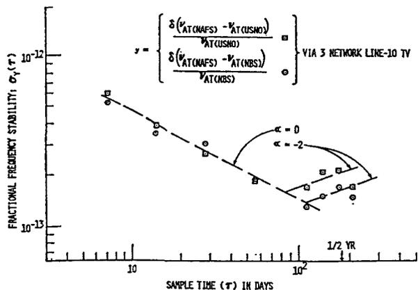
Fig. 6. Fractional frequency stability,  $\sigma_y(\tau)$ , of the Boulder-Newark and the Washington, D.C.-Newark paths via the 3-network TV line-10 technique
