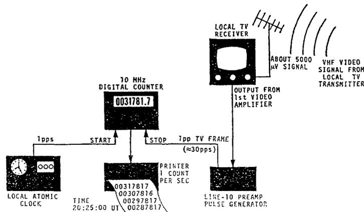
Fig. 2. Overview of receiving laboratory instrumentation for TV line-10 clock synchronization
