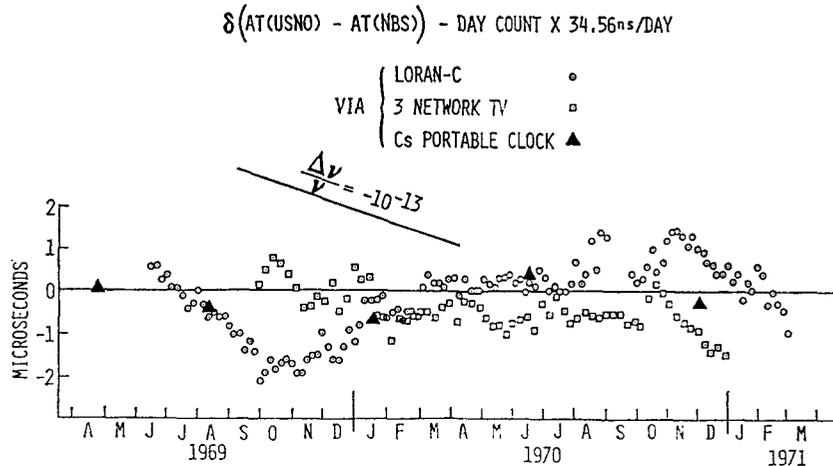
Fig. 5. Relative time differences of the AT(NBS) — AT(USNO) time scales compared by the Loran-C, 3-network TV line-10, and cesium portable clock techniques plus arbitrary constants
