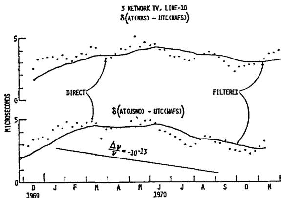
Fig. 7. Time differences (direct and filtered) of the Boulder-Newark and the Washington, D.C.-Newark paths via the 3-network TV line-10 technique plus an arbitrary constant
