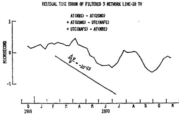
Fig. 8. Residual time differences of the 3-network TV line-10 technique between Boulder, Newark, and Washington, D.C.
