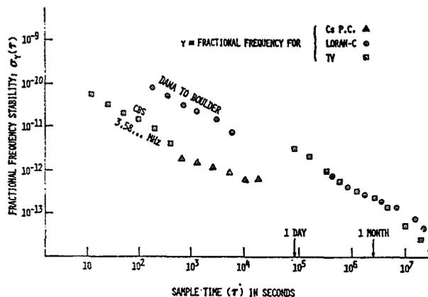
Fig. 11. Relative fractional frequency stability,  $\sigma_y(\tau)$ , versus sample time for Loran-C, 3-network TV line-10, CBS TV color subcarrier, and cesium portable clock
