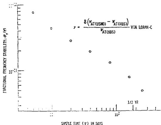
Fig. 9. Apparent Loran-C fractional frequency stability,  $\sigma_y(\tau)$ , over a continental USA path
