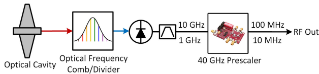
FIGURE 1. Block diagram of the optical-to-RF synthesis chain.
