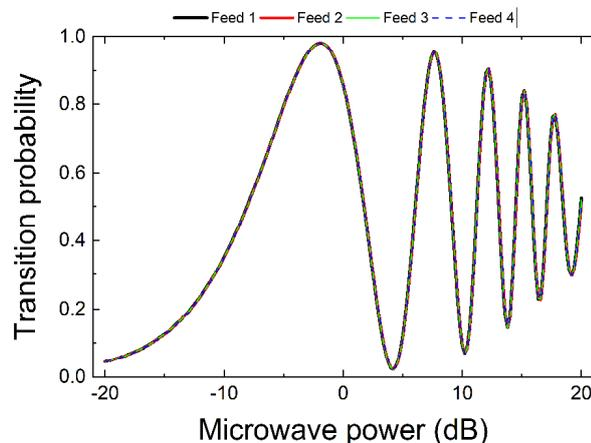
Figure 3. Transition probability as a function of microwave power for each individual feed after balancing each arm in the network by fine-tuning the attenuation. The maximum difference in transition probability between the four feeds shown is 0.027 over the full scan. Near normal operating power (first maximum), the transition probability due to individual feeds agree to better than 0.005.
