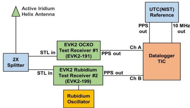
**Figure 1.** Configuration for comparing STL receiver timing to UTC(NIST).
