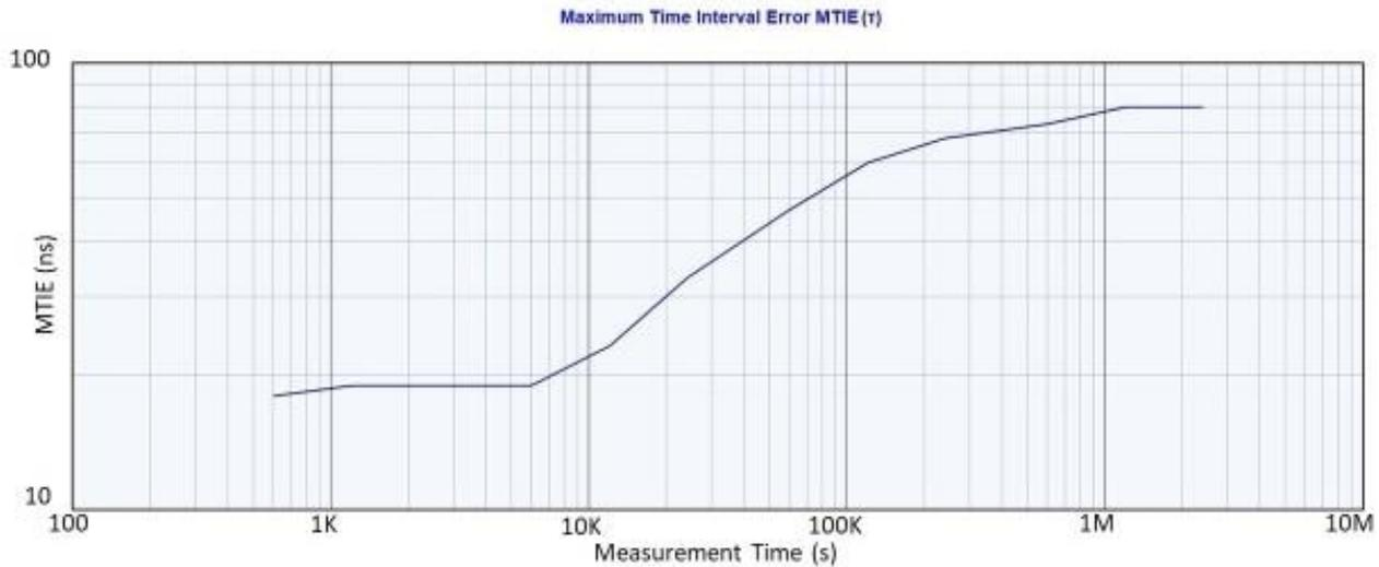
**Figure 3b.** STL rubidium receiver MTIE relative to UTC(NIST) for a 66-day period. The first data point is at 600 seconds because 10-minute average data is used.
