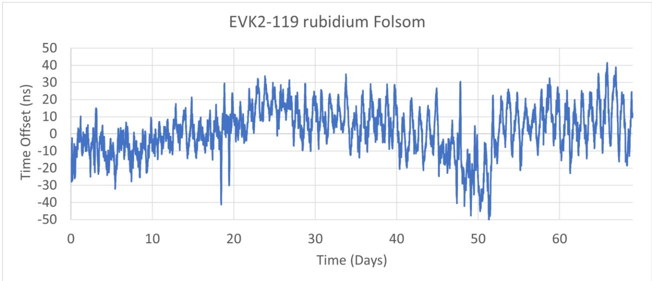
**Figure 6a.** STL rubidium receiver timing performance relative to GPS at Folsom lab over 69 days.
