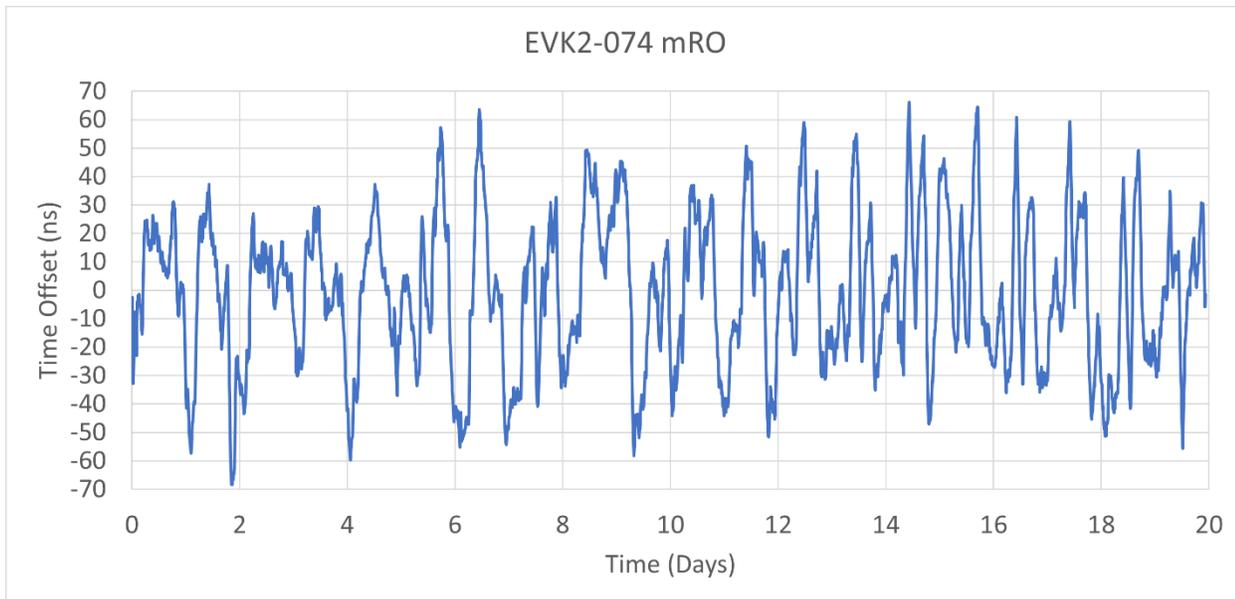
**Figure 11.** STL mini-rubidium receiver timing performance at Folsom lab over 20 days
