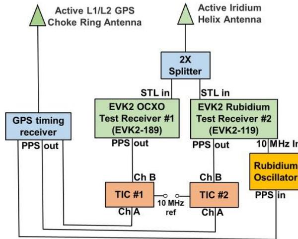
**Figure 4.** Configuration for measuring STL receiver timing error at Folsom lab.
