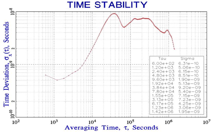
**Figure 8a.** Time stability (TDEV) of EVK2-199 Rb receiver with respect to UTC(NIST)
