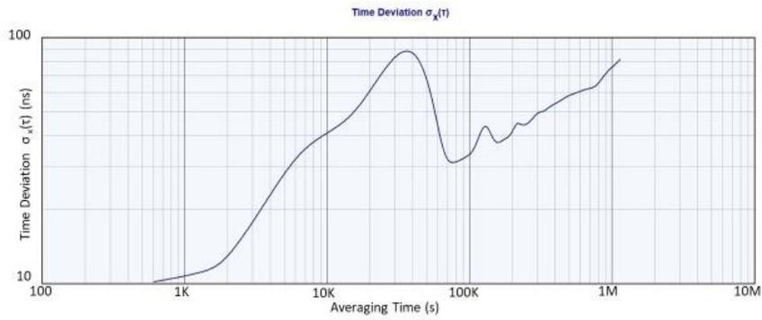
**Figure 8b.** Time stability of EVK2-119 receiver at Folsom lab with respect to GPS
