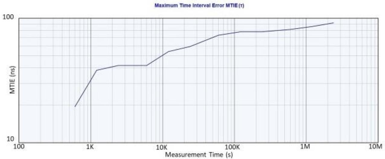
**Figure 6b.** STL rubidium receiver MTIE relative to GPS at Folsom lab over 69 days. The first data point is at 600 seconds because 10-minute average data is used.
