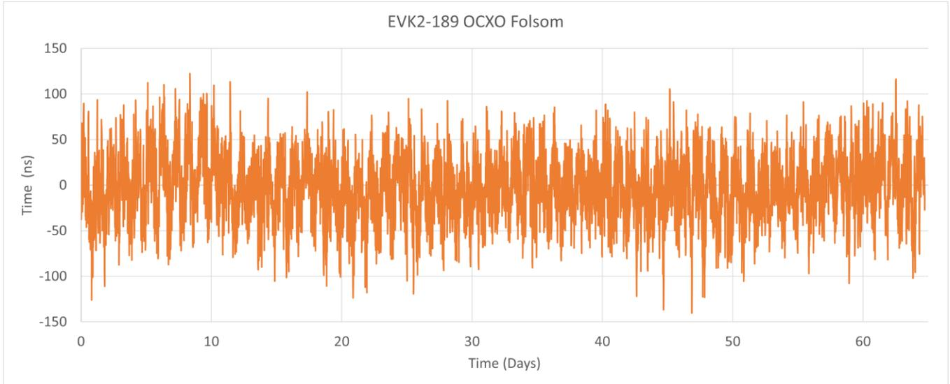
**Figure 5.** STL OCXO receiver timing performance relative to GPS at Folsom lab over 64 days.
