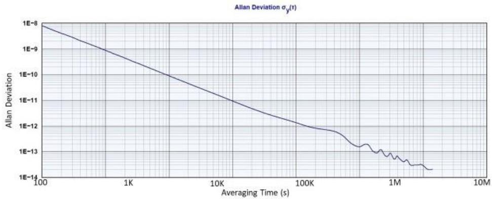
**Figure 9.** Stability (ADEV) of STL rubidium receiver with respect to GPS at Folsom lab
