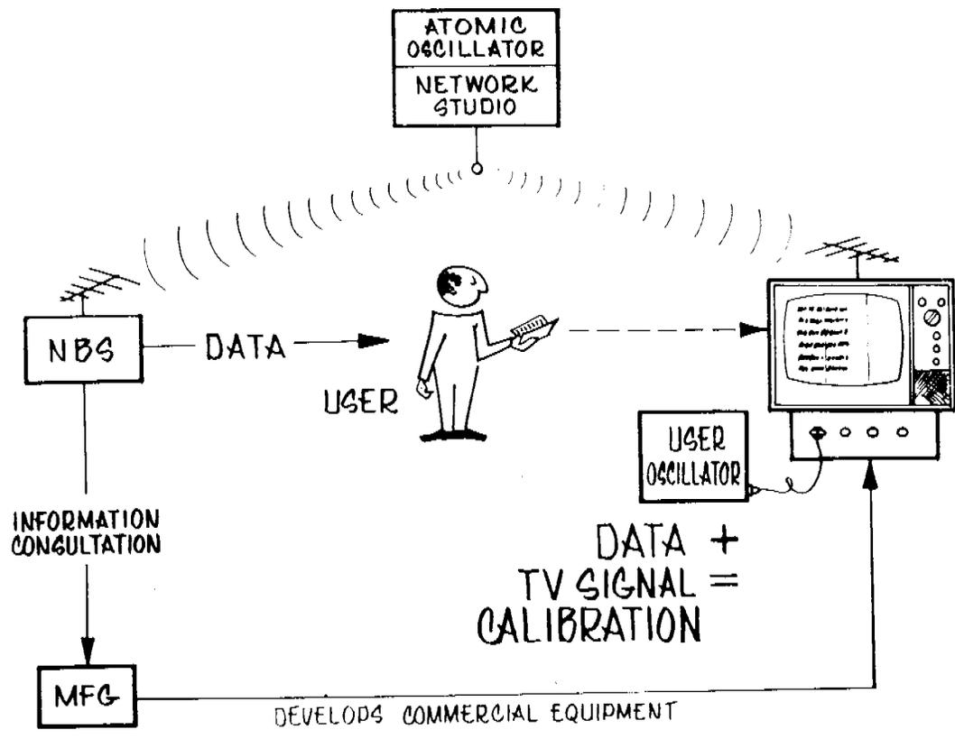
Fig. 6-TV frequency calibration service
