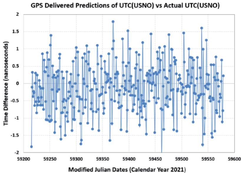
Figure 2. GPS delivered predictions of UTC(USNO) compared to actual UTC(USNO) for 2021.
