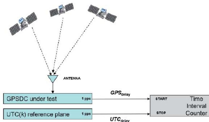
Figure 3. The GPSDC – UTC( $k$ ) time-difference measurement.
