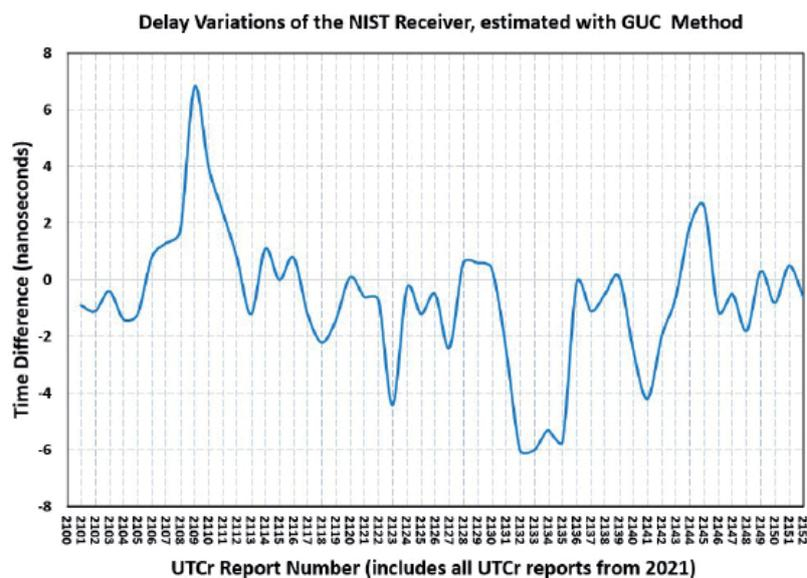
Figure 5. Post-calibration delay variations of the NIST receiver, estimated with the GUC method, for calendar year 2021.
