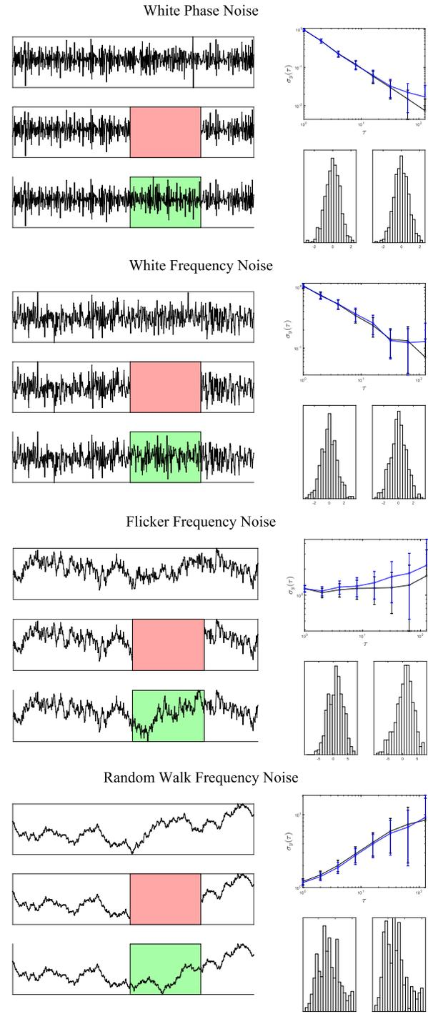
Fig. 3. Application of data imputation algorithm on simulated data of the four predominant noise types. Left: The data reconstruction algorithm. On the top left is the original data, in the middle left the dataset with values removed, and on the bottom left the dataset with imputed values. Top Right: The Allan deviations for the original (black) and recovered (blue) datasets. Bottom Right: The distribution for the original is in the left box and for the recovered data is in the right box.
