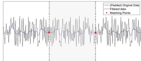
Fig. 7. Plot of the filtering function acting on the data. The middle section is the data segment, padded on either side of the gray dashed line with its own reflection. The thin blue line is then the filtered data with the two filtered are used for endpoint matching. Filtered points are highlighted by the dots in red.
