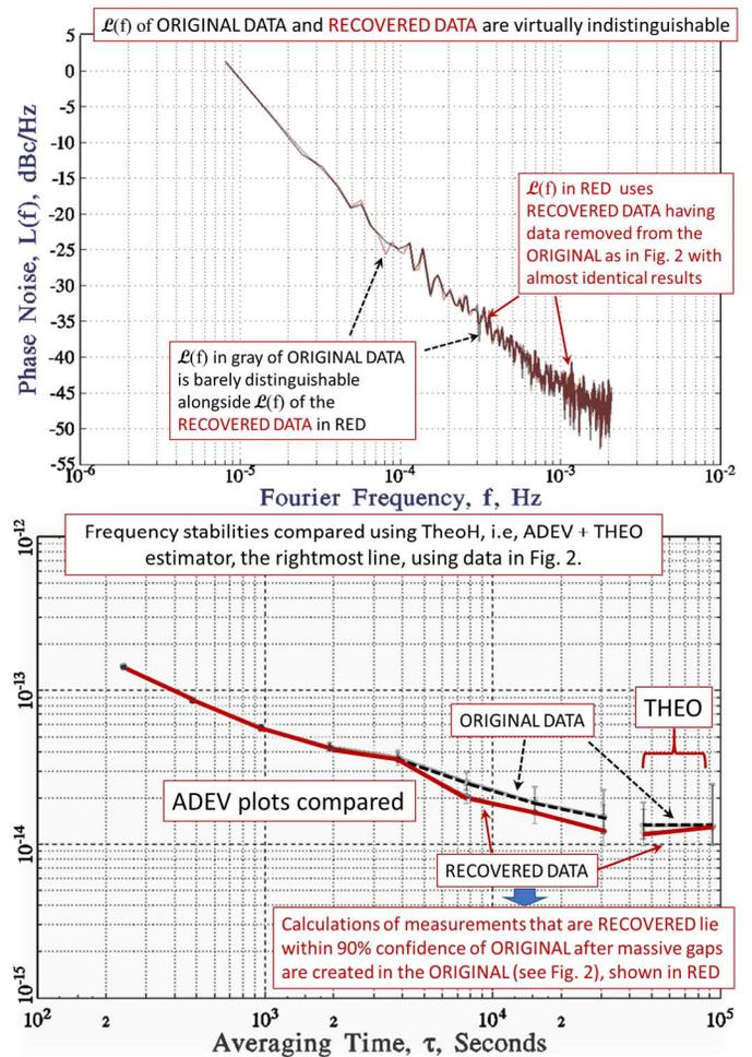
Fig. 3. TOP:  $\mathcal{L}(f)$  shows that original vs. recovered phase noise are virtually identical and that the recovered data extends to the same low Fourier frequency as the original. BOTTOM: Frequency stability using high-confidence TheoH of original vs. recovered data.
