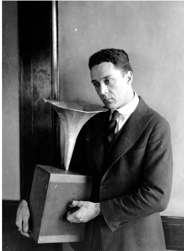
Fig. 7. Portaphone portable receiver, 1921.
