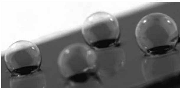
FIG. 16. Micro-glassblown alkali vapor cells. Reprinted with permission from E. J. Eklund et al. , Sens. Actuators A 143 , 275–280 (2008). Copyright 2008 Elsevier.
