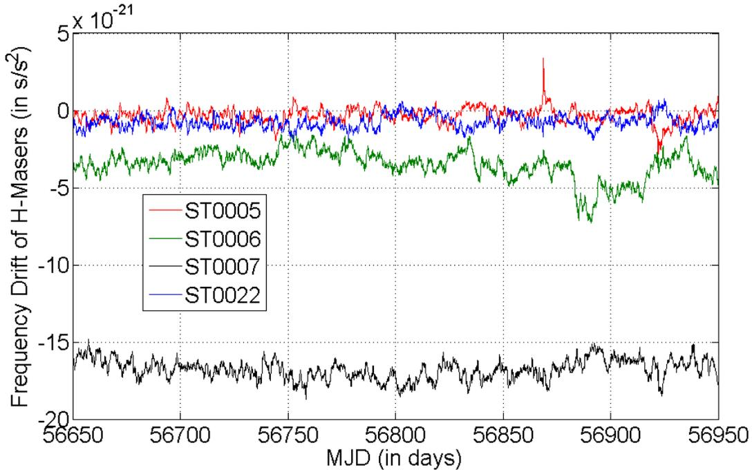
**Figure 2.** Frequency drift of H-masers.
