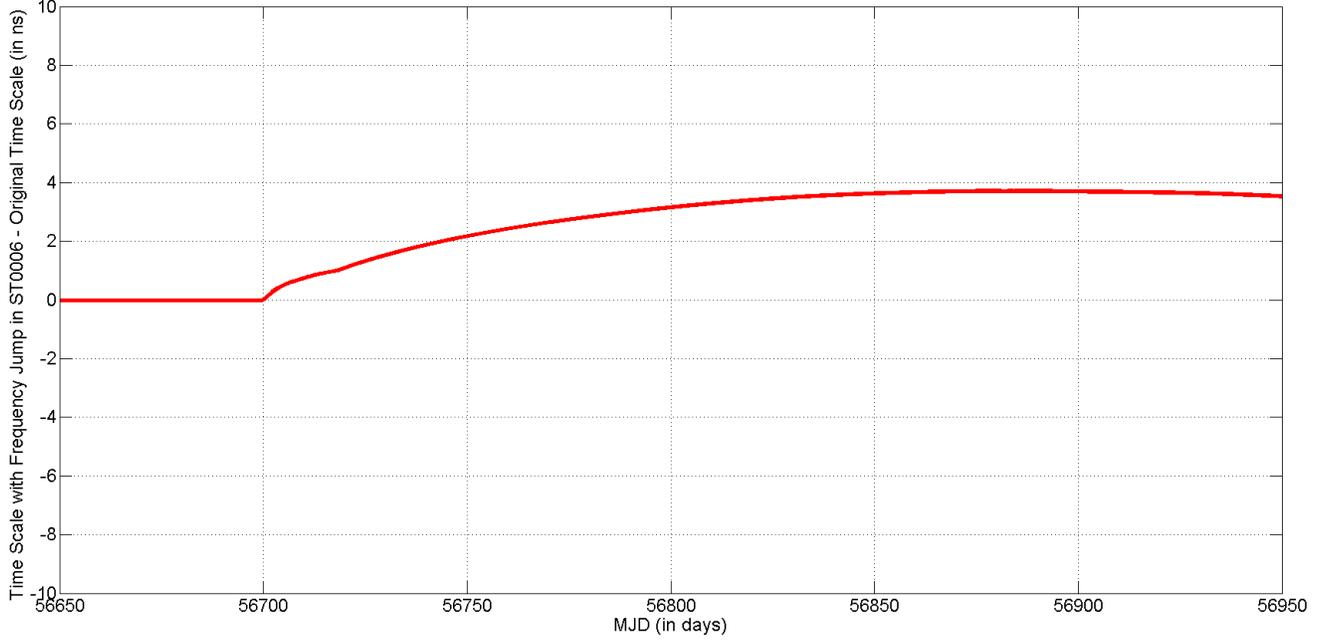
**Figure 4.** Response of the time scale to a frequency jump. We artificially add a frequency jump of  $6.8 \times 10^{-15}$  s/s in ST0006 at MJD 56700.0.
