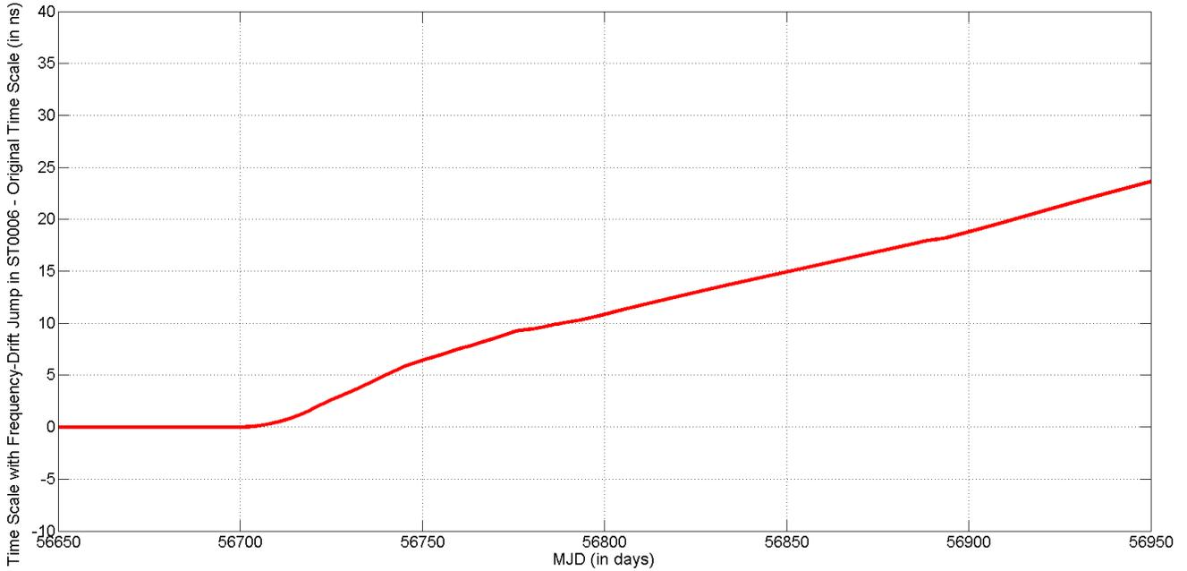
**Figure 5.** Response of the time scale to a frequency-drift jump. We artificially add a frequency-drift jump of  $5.36 \times 10^{-21}$  s/s<sup>2</sup> in ST0006 at MJD 56700.0.
