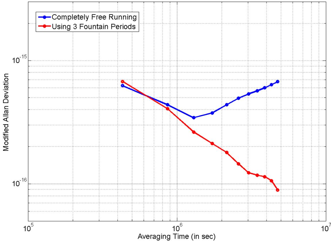
**Figure 7.** The frequency stability of the time scale using three fountain periods (red curve), versus the frequency stability of the free-running time scale (blue curve).
