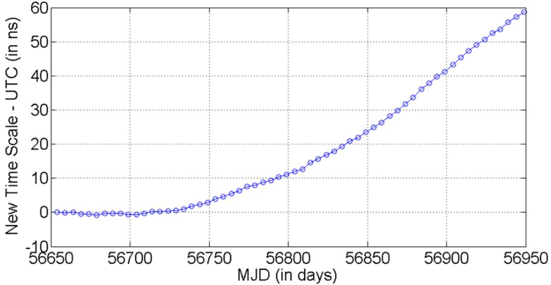
**Figure 1.** Free-running Kalman-filter H-maser time scale with respect to UTC.
