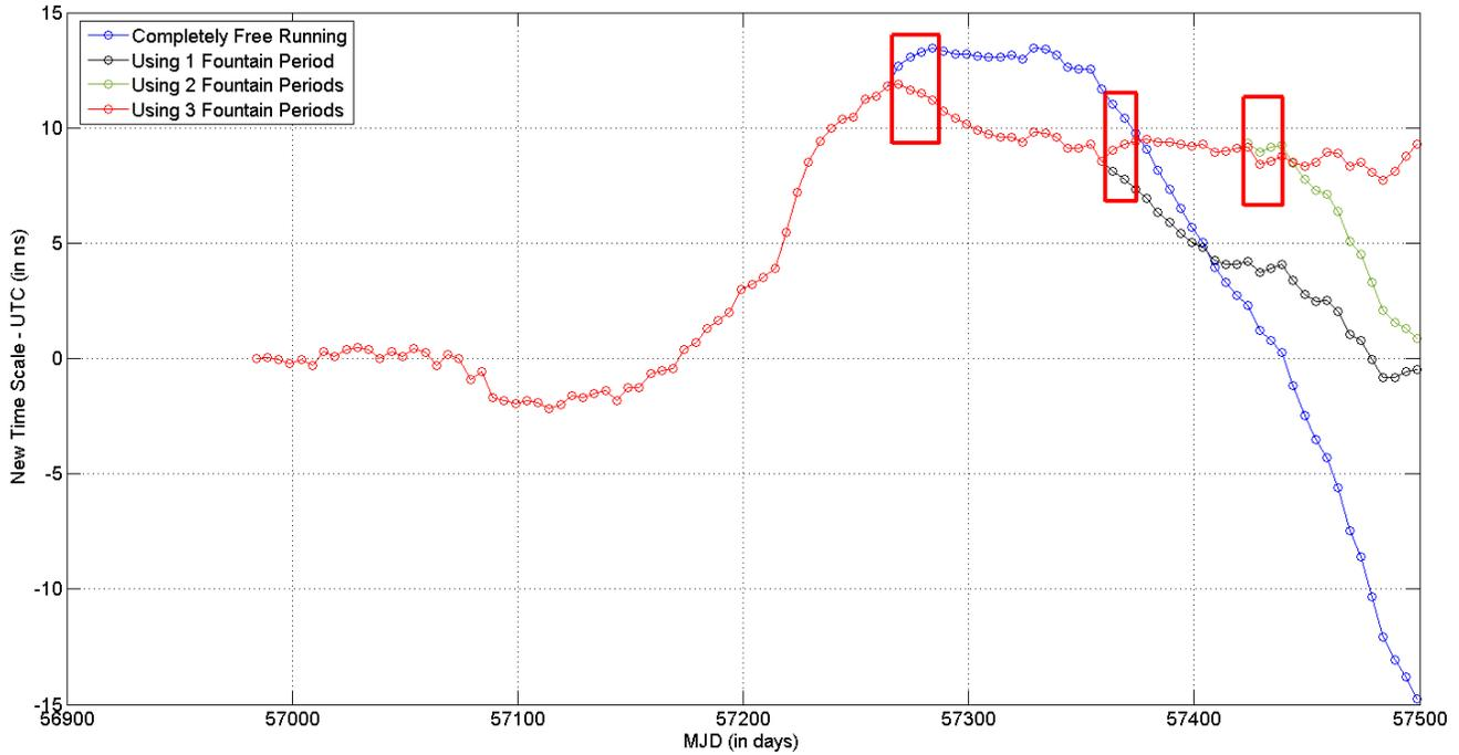
**Figure 6.** Steering the free-running time scale to the NIST F1 Cs fountain. Note, the blue curve is the same as the red curve during MJD 56980.0 – 57264.9; the black curve is the same as the red curve during MJD 56980.0 – 57360.0; the green curve is the same as the red curve during MJD 56980.0 – 57420.8.
