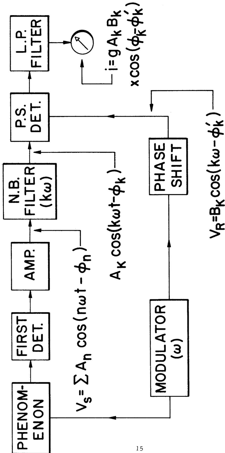
Figure 1. Block Diagram of Conventional Mode
