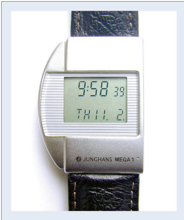
Fig. 4. Junghans MEGA 1, the first radio controlled wristwatch.
