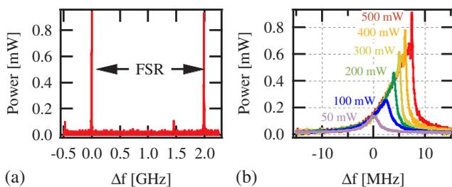
FIG. 2 (color online). (a) The laser is tuned across a cavity FSR. Slight polarization rotation reveals the birefringent mode shifted by  $\sim 500$  MHz. (b) Thermal runaway as the pump laser is tuned through cavity resonance.
