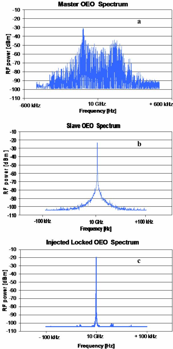
Figure 2. RF Spectrum of (a) Master OEO, (b) Slave OEO and (c) Injection Locked OEO at 10 GHz.
