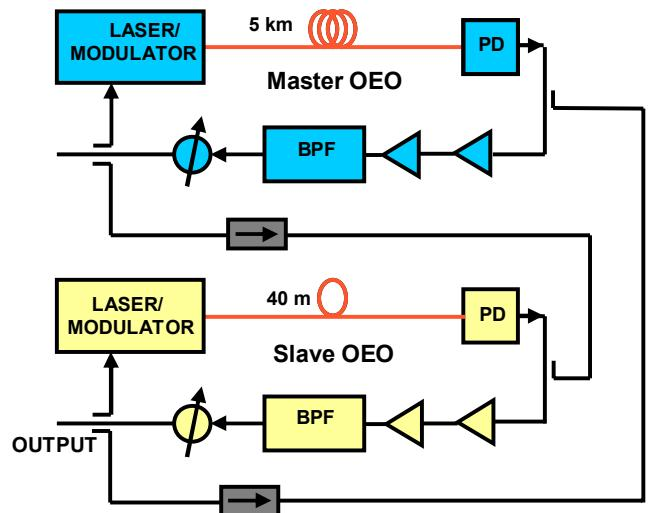
Figure 1. Block diagram of a dual-fiber, injection-locked optoelectronic oscillator (DFIO). PD: photo detector; BPF: bandpass filter.
