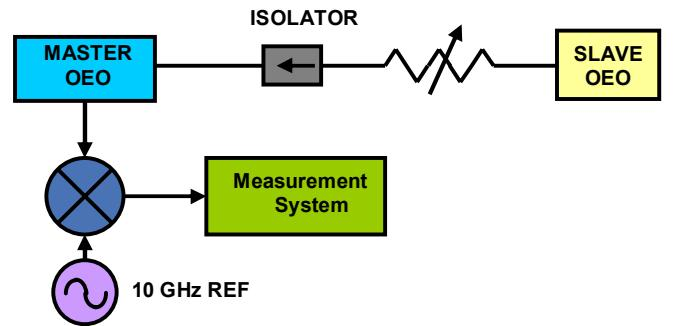
Figure 5. Experimental setup of the master OEO injection locked to the slave OEO.
