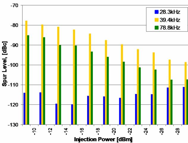
Figure 10. Graph showing the spurious levels as a function of master-to-slave injection.
