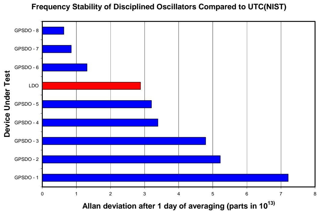
Figure 8. A comparison of LDO frequency stability to eight different GPSDOs.
