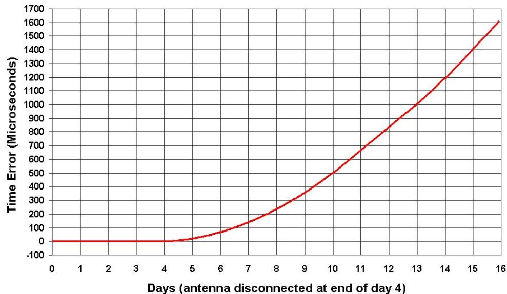
*Figure 5. Phase plot of rubidium GPSDO with poor holdover capability during simulated signal outage.*
