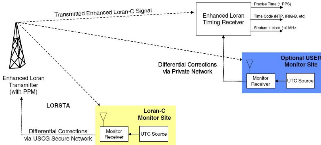
Figure 9. USCG monitoring sites provide the differential corrections included in eLORAN broadcasts.
