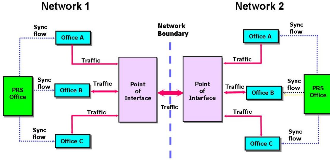
*Figure 1. A plesiochronous connection between two networks. Each network maintains its own PRS.*
