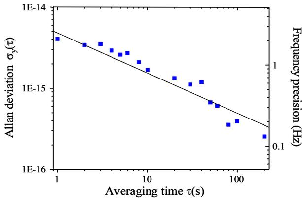
Figure 8. Allan deviation (squares) of the effective beatnote between the Yb and Ca standards. Shown for reference is a line corresponding to an Allan deviation of  $5 \times 10^{-15} \tau^{-1/2}$ .
