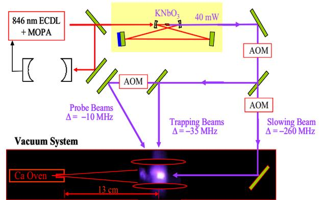
Figure 2. The trapping apparatus for the Ca clock. Omitted for clarity is a Zeeman magnet coil between the oven and the trap center.
