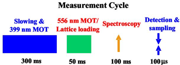
Figure 6. The measurement cycle for the Yb lattice clock. The lattice light remains on throughout the entire cycle. The spectroscopy period ranges from 1 ms at low resolution to 200 ms for high resolution.
