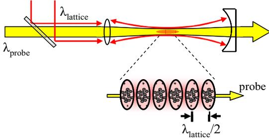
Figure 5. Lattice apparatus showing the 1-D horizontal standing wave and the co-propagating single-pass probe. Roughly 10-20 atoms are contained in each pancake-like potential well.
