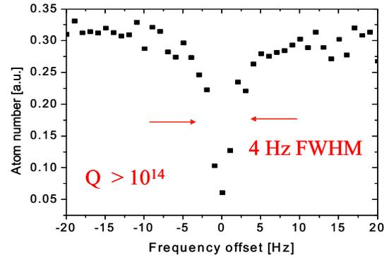
Figure 7. High resolution spectroscopy of the Yb clock transition. Excitation leads to a depletion of the ground state population as measured by a near-resonant 399 nm detection pulse.
