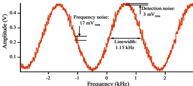
Figure 3. (Un-modulated) Bordé-Ramsey signal from the Ca spectrometer.
