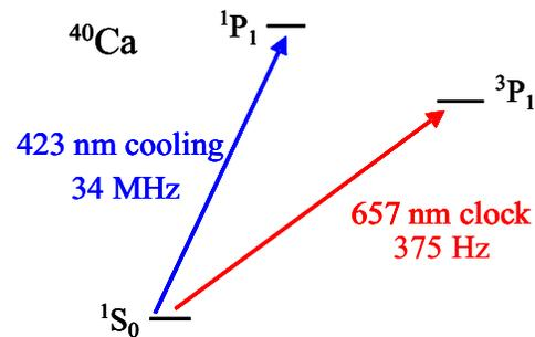
Figure 1. Relevant energy levels for the Ca optical clock
