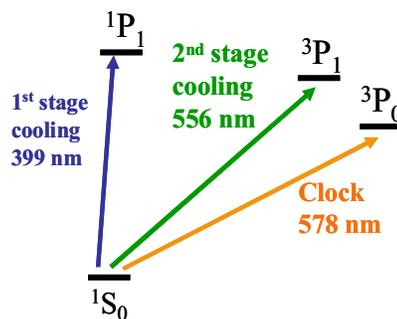
Figure 4. Relevant energy levels for the Yb lattice clock.
