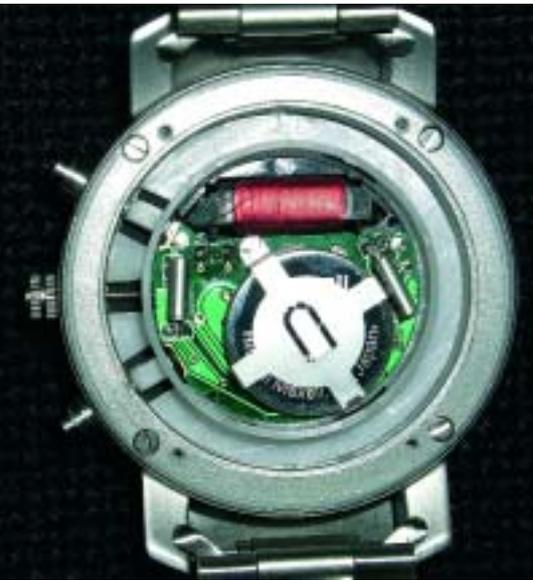
2. Rear view inside of a low-cost RCW, with two crystals and the antenna visible.
