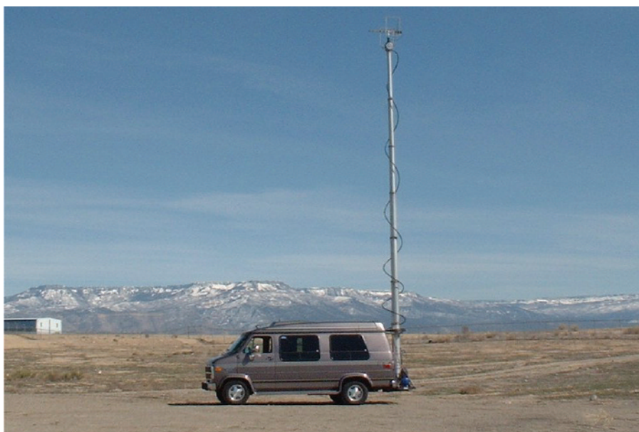
Figure 3. A mobile calibration van that tests whether or not a transmitter is within tolerances specified by the FCC (courtesy of dbK Communications, Inc.).
