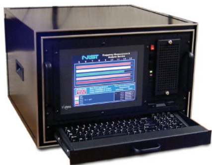
Figure 6. The measurement system supplied to subscribers to the NIST Frequency Measurement and Analysis Service. It makes frequency measurements traceable to the NIST standard by using GPS as a transfer standard.
