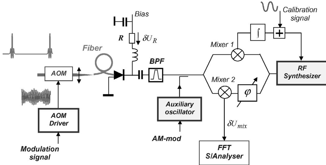
Fig. 3. Experimental setup for measurement of power-to-phase conversion in photodetectors.
