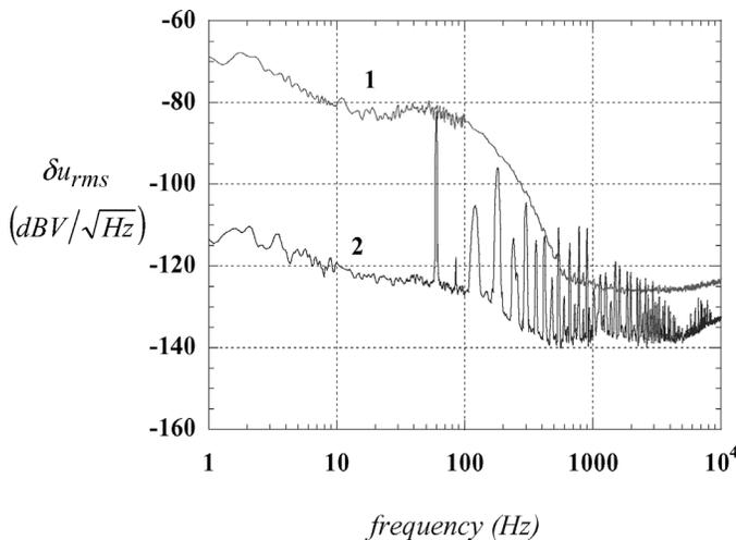
Fig. 10. Spectra of voltage fluctuations across the load resistor of a photodetector used as sensor for the control system stabilizing average power of the femtosecond pulse train: feedback loop is open (curve 1), feedback loop is closed (curve 2).
