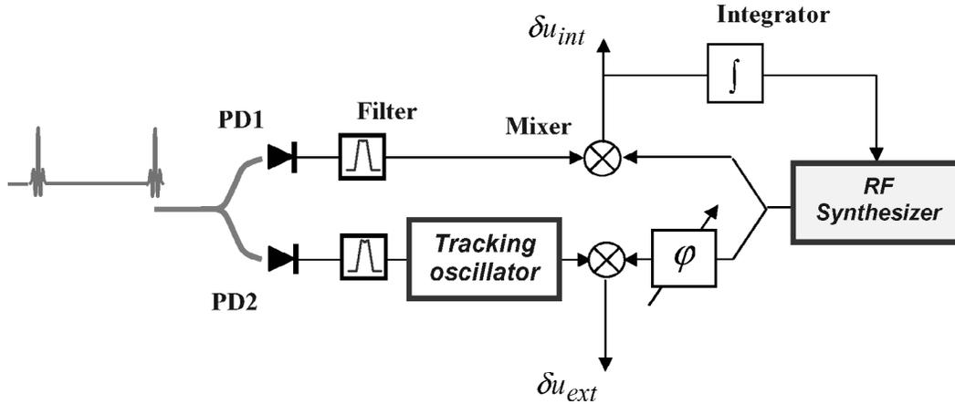
Fig. 7. Schematic of a dual-channel read-out system for measuring the excess phase noise associated with demodulation of ultra-short light pulses.
