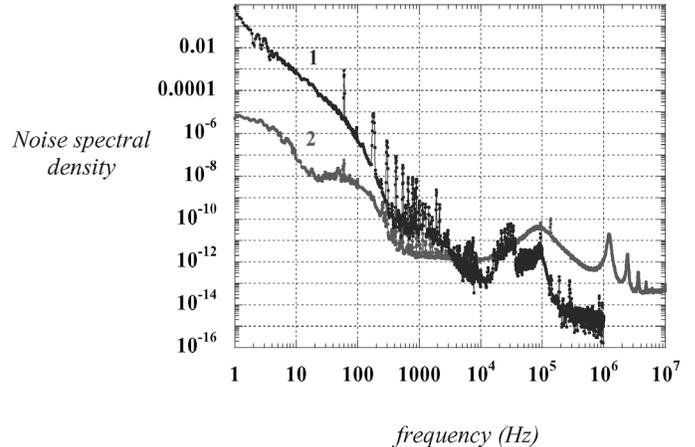
Fig. 2. Spectra of phase (curve 1) and amplitude (curve 2) fluctuations of a signal at second harmonic of pulse repetition rate at the output of a photodetector illuminated with a Cr: forsterite femtosecond laser. The units of the vertical axis are  $\text{rad}^2/\text{Hz}$  for the phase noise and  $1/\text{Hz}$  for the amplitude noise, respectively.
