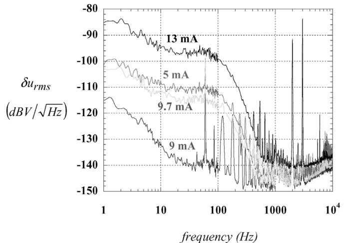
Fig. 8. Spectra of voltage fluctuations at the output of the external channel of the dual-channel phase sensitive read-out system at different levels of photocurrent. Measurements were carried out with two “Discovery” photodetectors at the frequency 866 MHz which is the second harmonic of pulse repetition rate. Bias voltages were set to 6 V, the load resistances were 100 ohm.
