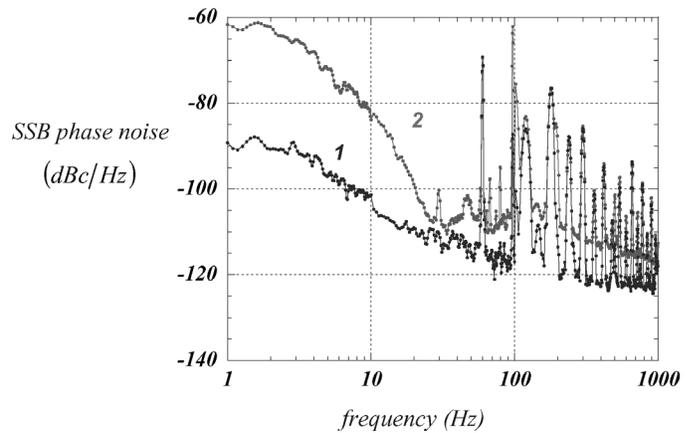
Fig. 11. Effect of power control system on the excess phase noise in the spectrum of the second harmonic of pulse repetition rate: control system is activated (curve 1), control system is off (curve 2). Photocurrent is 11.4 mA.
