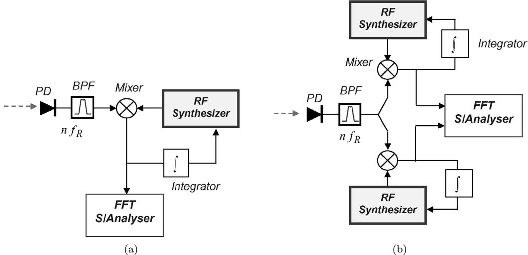
Fig. 1. Single-channel (a) and dual-channel (b) two oscillator phase noise measurement systems.
