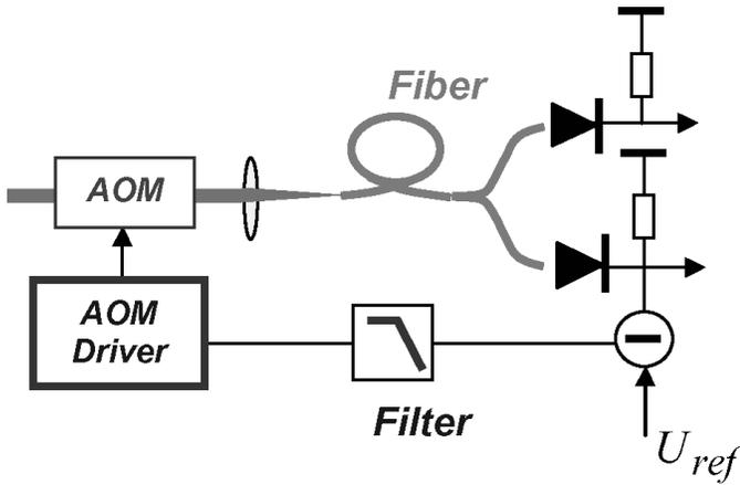
Fig. 9. Schematic of laser power stabilization system.
