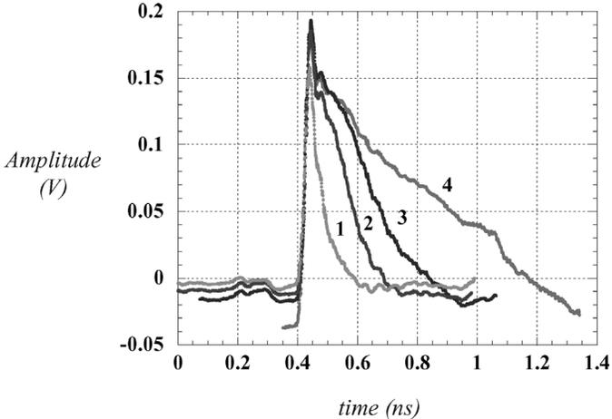
Fig. 6. Demodulated light pulses at the output of “Discovery” photodetector at different levels of optical power (photocurrent): curve 1, photocurrent  $I_{DC} = 1.1$  mA; curve 2, photocurrent  $I_{DC} = 3$  mA; curve 3, photocurrent  $I_{DC} = 5$  mA; curve 4, photocurrent  $I_{DC} = 11$  mA. Photodetector is directly connected to a matched input of a high-speed oscilloscope.
