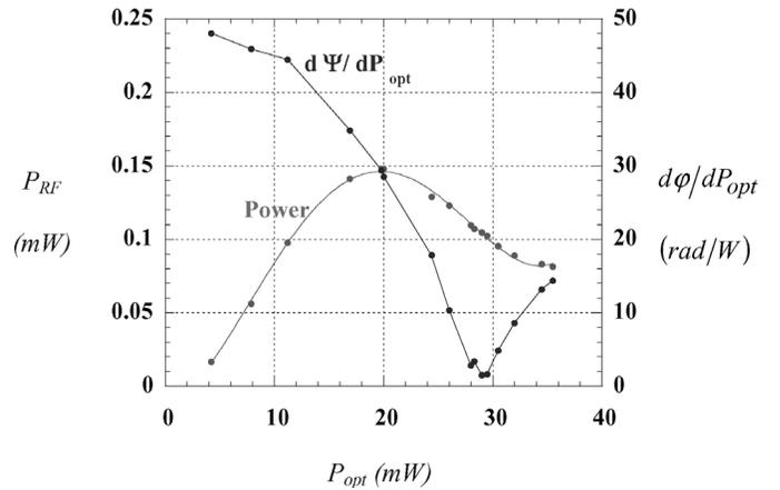
Fig. 4. Power of second harmonic of pulse repetition rate (866 MHz) and power-to-phase conversion at the same frequency as a function of average power of the optical comb. “Discovery” photodetector, load resistor 100  $\Omega$ , bias voltage 6 V.
