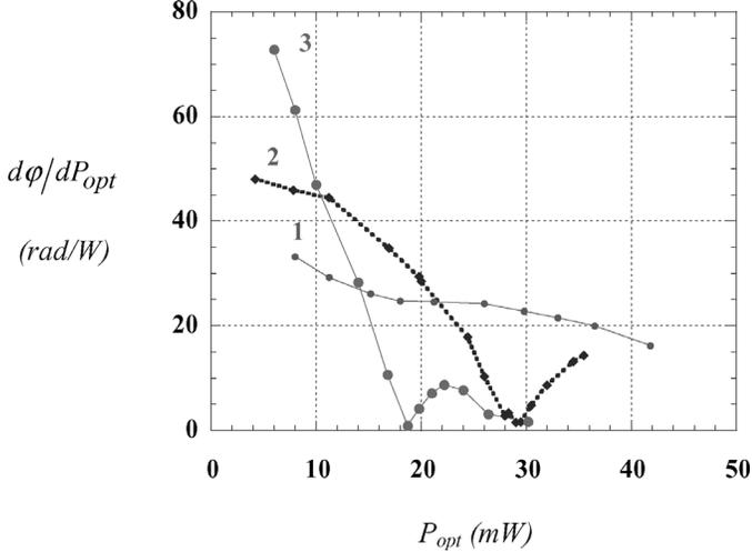
Fig. 5. Power-to-phase conversion at different harmonics of pulse repetition rate as a function of average power of the optical comb: curve 1 is for 433 MHz, curve 2 is for 866 MHz, curve 3 is for 1299 MHz.
