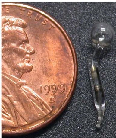
Fig. 1. (Color online) Cs-vapor microcell, whose inner walls are coated with paraffin, used for the present measurements.
