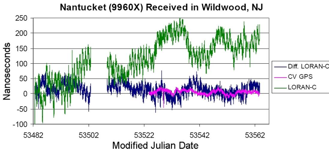
Figure 3. Comparison of Legacy LORAN-C and Differential LORAN-C for Time Recovery.
