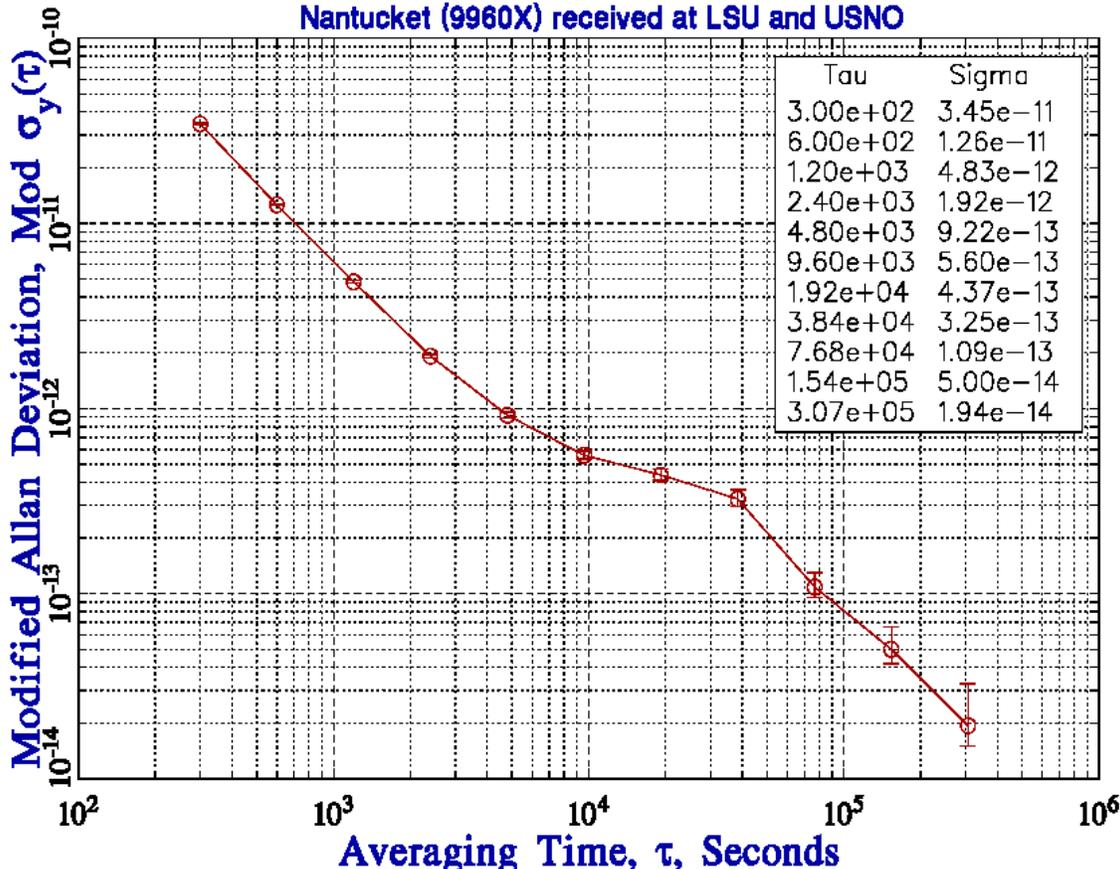
Figure 5. Frequency stability of LORAN-C with corrections applied from monitor sites..
