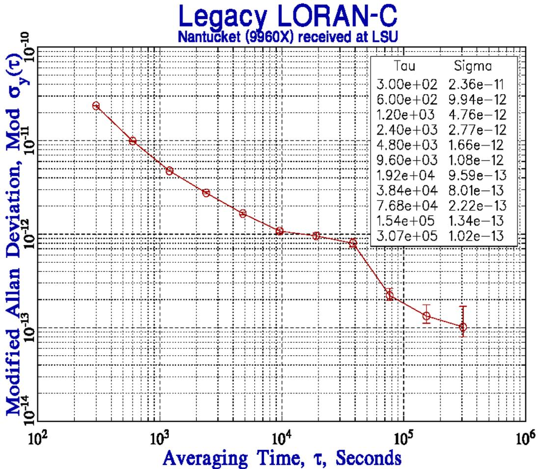
Figure 4. Frequency stability of legacy LORAN-C.
