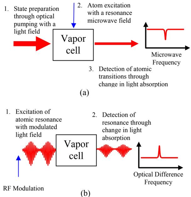
Figure 2 Physical mechanisms involved in (a) conventional microwave-excited vapor cell frequency references and (b) frequency references based on coherent population trapping.
