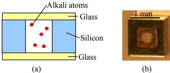
Figure 3 (a) Basic MEMS cell geometry (side view) and (b) photograph of millimeter-scale cells made at NIST in 2003 (top view).
