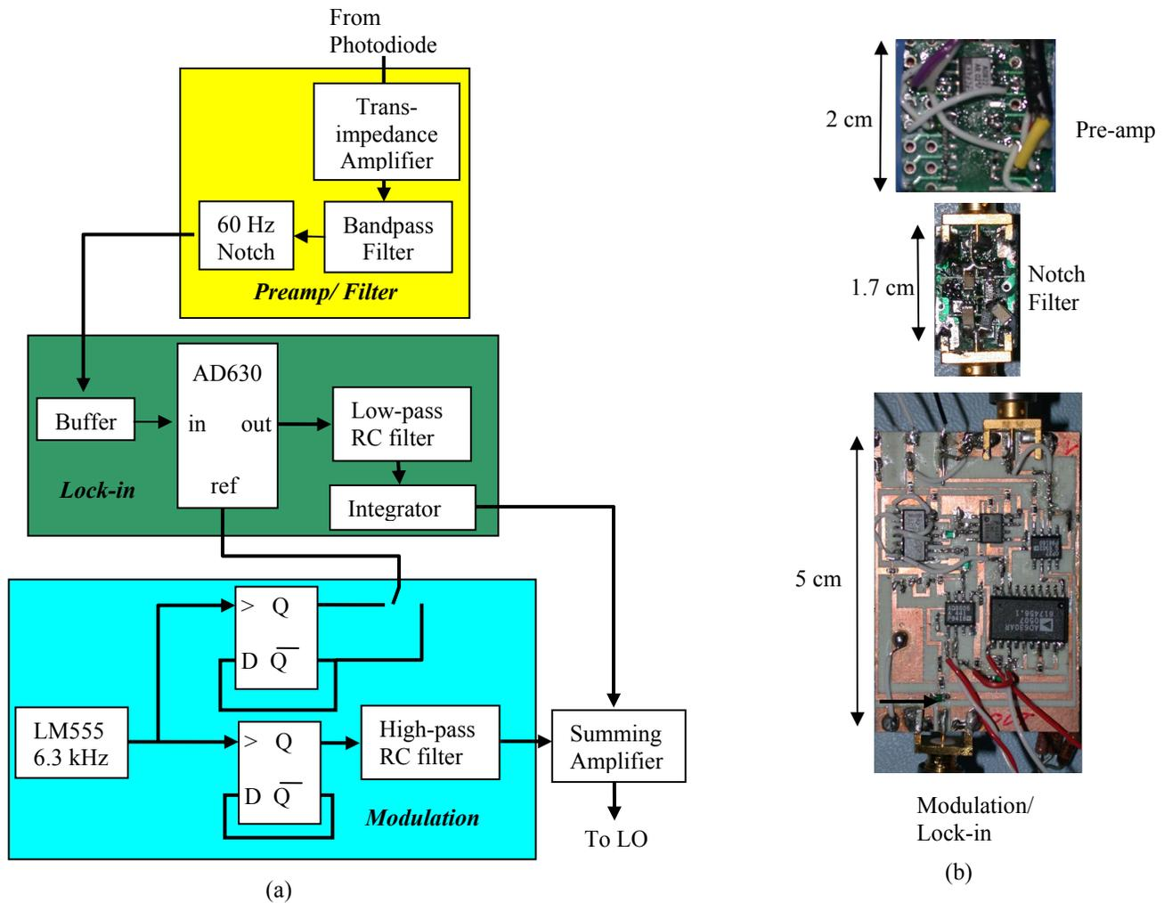
Figure 6 (a) Schematic and (b) Photographs of control electronics used to lock the frequency of the local oscillator to the atomic transition resonance generated by the physics package.
