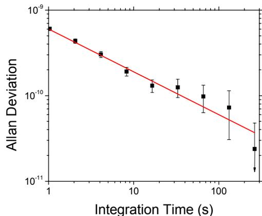
Figure 8 Allan deviation of low-power LO when locked with the compact control electronics to the MEMS physics package. A fractional frequency stability of  $6 \times 10^{-10}/\sqrt{\tau}$  is obtained for  $0 < \tau < 100$  s.
