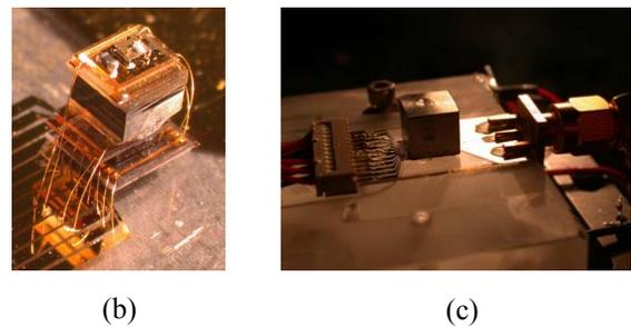
Figure 4 Physics package for a chip-scale atomic clock. (a) Schematic of the shielded physics package. (b) Photograph of the (unshielded) package and (c) photograph of the shielded unit.
