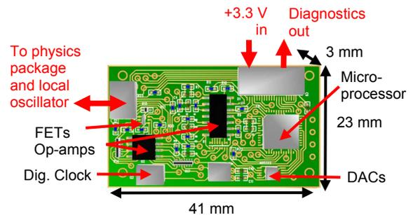
Figure 7 Digital control system under development to replace the analog system shown in Figure 6.
