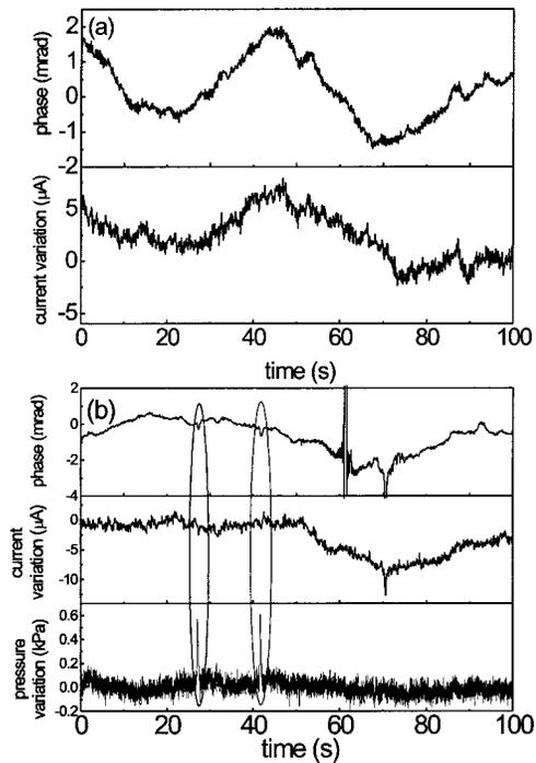
Fig. 2. (a) Phase between two 10-GHz signals derived from a common optical reference at equal  $f_{R,i}$  (upper trace) and variation of the photocurrent through one of the photodetectors from its mean value (lower trace). (b) Upper and middle trace show data as in (a), and the lower trace depicts variations of ambient pressure from the mean value. Ellipses mark times when a laboratory door was opened. At 61 and 70 s the system was deliberately perturbed.
