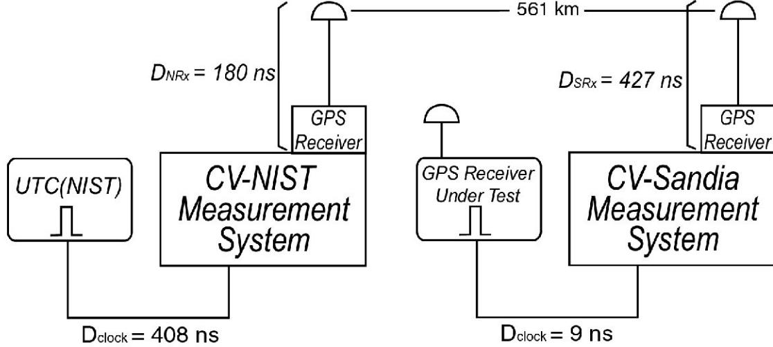
Figure 5. Block diagram of comparison with delay values entered.
