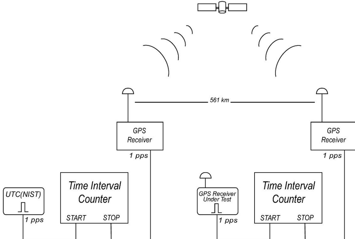
Figure 4. Common-View GPS Measurement Configuration.
