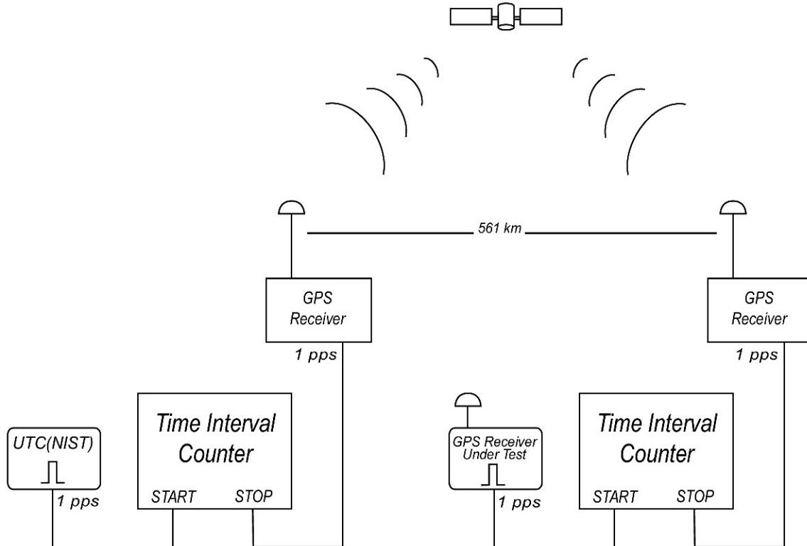
Figure 4. Common-View GPS Measurement Configuration.
