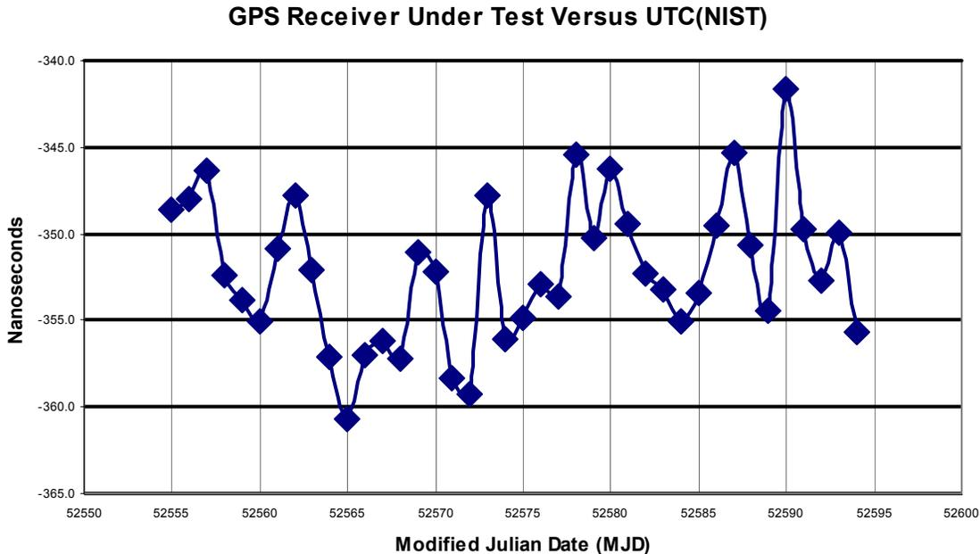
Figure 6. Results of 40-day remote calibration of GPS timing receiver.
