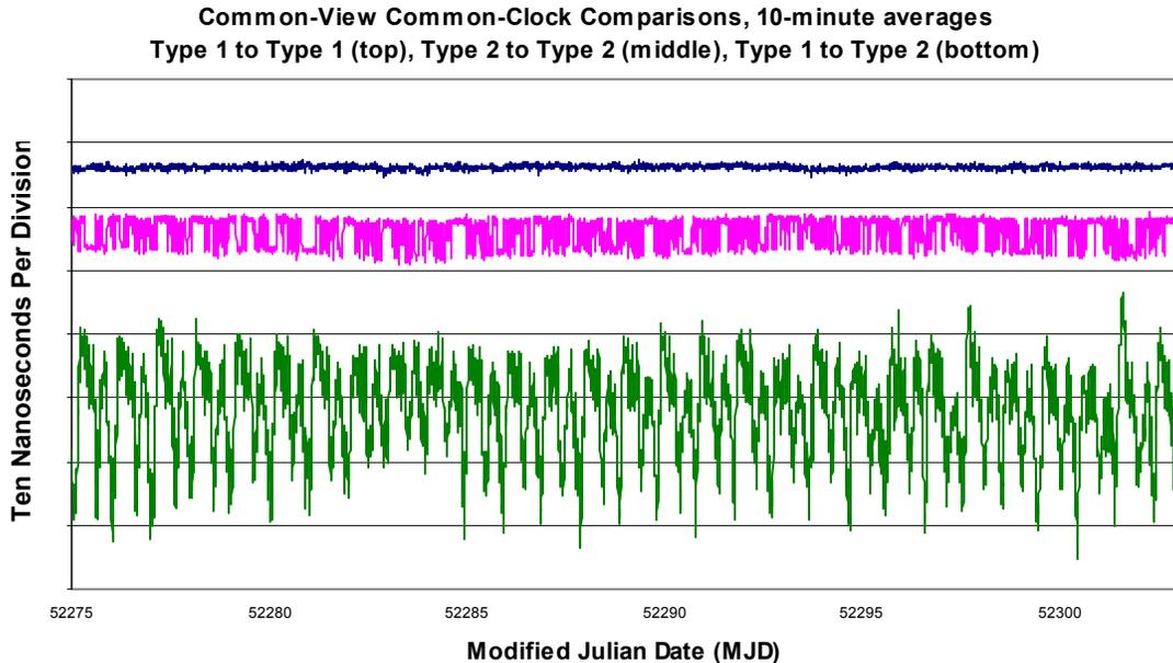
*Figure 3. Results of Common-Clock Comparison using two different receivers.*
