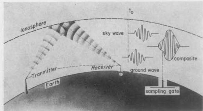
Fig. 2—Ground wave resolution with Loran-C.
