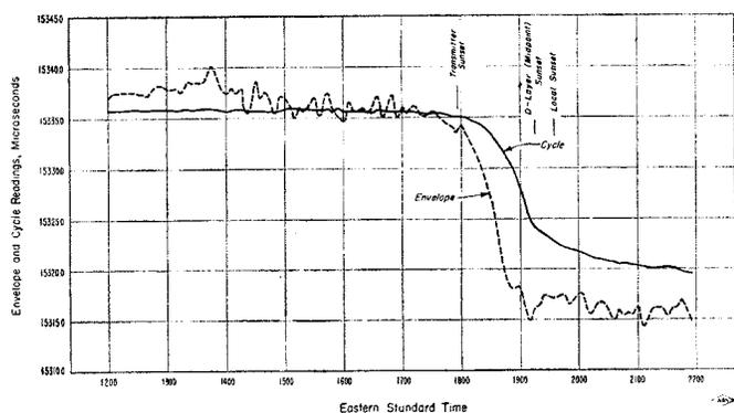
Fig. 31—First-hop sky wave measurements—Boulder, Colo. (October 6, 1955).
