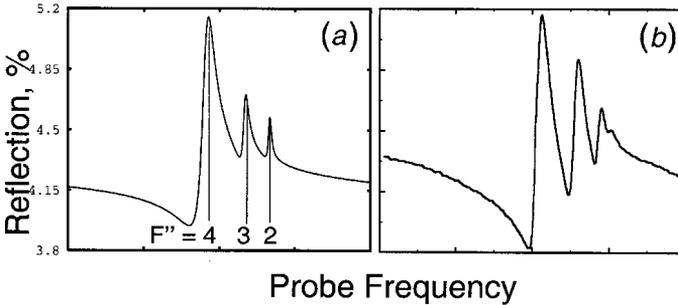
Figure 4. Calculated (a) and experimental (b) selective reflection spectrum when the probe frequency is swept in the area red shifted ( $\sim 800$  MHz) from the D<sub>2</sub> line of  $^{87}\text{Rb}$  ( $F = 2 \rightarrow F'$ ). The drive frequency is fixed and tuned to the  $5P_{3/2}$ ,  $F' = 3 \rightarrow 5D_{5/2}$  transition of  $^{87}\text{Rb}$ . Observed resonances correspond to the fine structure of the  $5D_{5/2}$  state. Incident angle is equal to  $\alpha = 0.1$  rad.
