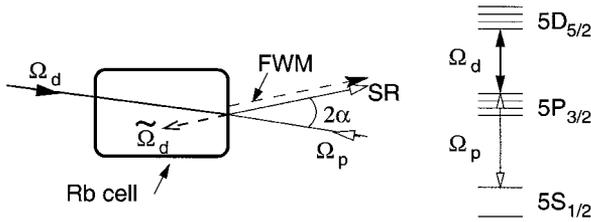
Figure 1. Experimental set-up and scheme of atomic levels.
