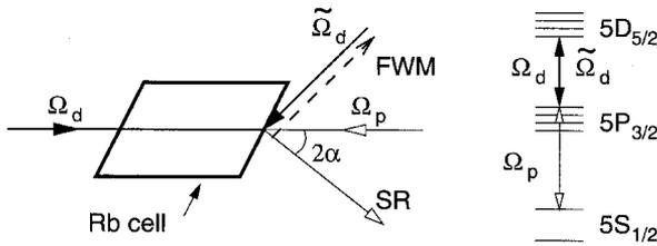
Figure 2. Experimental set-up to study four-wave-mixing process on the interface between glass and rubidium vapour.
