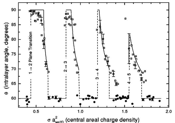
FIG. 7. Intralayer angle  $\theta$  structure as a function of normalized areal charge density. The lines are the predictions of theory, and the symbols are experimental measurements. Representative error bars are included with some of the measurements.
