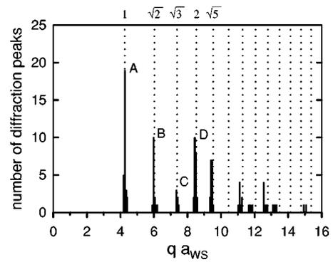
FIG. 3. Histogram showing the numbers of peaks (not intensities) observed as a function of  $q \cdot a_{\text{WS}}$  (defined in the text) for 30 time-averaged Bragg scattering patterns obtained on two different spherical plasmas with  $N > 2 \times 10^5$ . The dotted lines show the expected peak positions for a bcc crystal, normalized to the center of gravity of the peak at A (corresponding to Bragg reflections off  $\{110\}$  planes). From Ref. 20.
