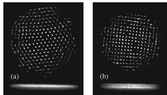
FIG. 5. Strobed top-view images of a small ( $N \sim 300$ )  $\text{Be}^+$  ion plasma phase-locked with a rotating dipole field at (a)  $\omega_r = 2\pi \times 65.7\ \text{kHz}$  and (b)  $66.5\ \text{kHz}$ . Below are unstrobed side views showing the axial lattice planes. Heavier-mass ions are located outside the  ${}^9\text{Be}^+$  ions.
