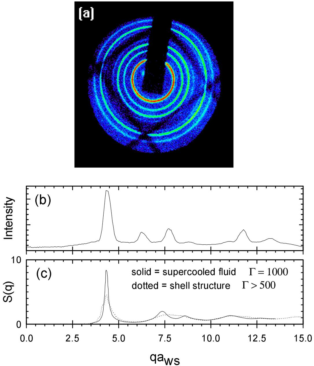
**Figure 2.** (a) Bragg scattering pattern observed from  $2.7 \times 10^5$  ions showing the presence of a crystal(s). The diffraction pattern is partially blocked by a rectangular shadow due to the laser beam deflector and a square shadow due to a wire mesh. (b) Differential cross-section obtained from an azimuthal average of (a) about the z-axis. © Fluid-like  $S(q)$  calculated for a super-cooled OCP and an  $N=5 \times 10^3$  ion cloud with shells.<sup>20</sup>
