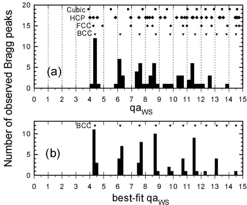
**Figure 3.** The number of observed peaks (not intensity) from 14 diffraction patterns with  $N=2.7 \times 10^5$  ions. In (a) there are no adjustable parameters ( $a_{ws}$  is determined from the observed  $\alpha$ ). In (b),  $a_{ws}$  is determined by fitting the diffraction patterns used in (a) to a bcc lattice. The ticks indicate the location of Bragg peaks for the simple cubic, hcp, fcc, and bcc lattices.
