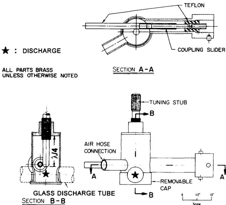
FIG. 1. Quarter-wavelength coaxial cavity operating at 2450 MHz. (Cavity 5 from reference [1].) The discharge location is shown with a star in the lower views.
