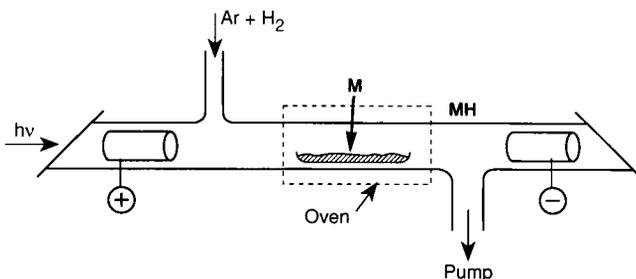
FIG. 5. Apparatus for the generation of metal hydrides by flowing discharged H<sub>2</sub> over metal heated in a furnace indicated by the dashed outline.
