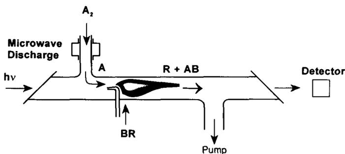
FIG. 4. A schematic diagram of the discharge/flow apparatus for the generation of short-lived molecules. The products of a discharge through flowing gas, producing A, are mixed with a continuous flow of a secondary gas BR and react downstream to generate the desired product.
