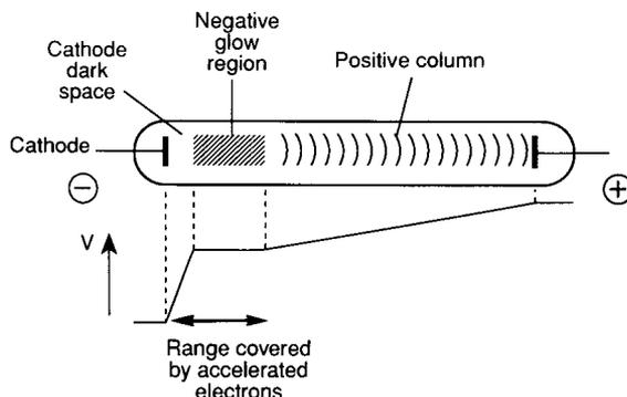
FIG. 2. A diagram showing the different regions in an electric discharge through a low pressure gas. The potential varies nonuniformly through the discharge as shown, the largest fall occurring in the cathode dark space. Positive ions are formed predominantly in the negative glow region.
