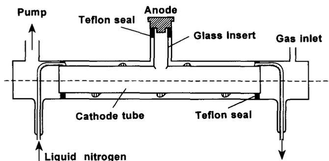
FIG. 3. A hollow cathode discharge cell for the generation of positive ions, after the design of van den Heuvel and Dymanus [8]. The copper cathode first inside a glass cell and is cooled by flowing nitrogen through a spiral tube soldered to its outside surface.
