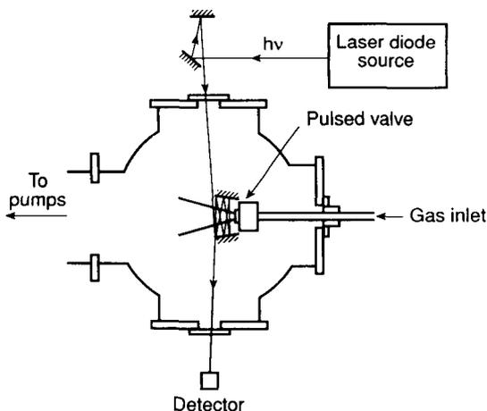
FIG. 6. Apparatus for the study of infrared spectra of van der Waals molecules, formed by supersonic expansion of the component gases through a pulsed nozzle. The system of tilted plane mirrors causes the laser beam to make several passes through the sample, thereby increasing the absorption.
