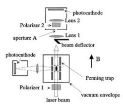
FIG. 1. Schematic diagram (not to scale) for detection of Bragg scattering from an ion cloud, shown as a small prolate spheroid, inside a Penning trap. An f/5 imaging system (left) monitors the shape of the cloud, thereby giving the ion density. The diffraction pattern is relayed to the upper photocathode, filtered by a small aperture (A) and crossed polarizers, as described in the text.
