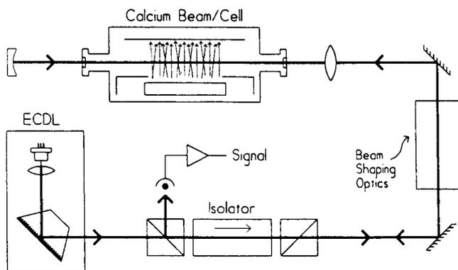
**Fig. 1.** Saturated-absorption spectrometer for calcium. The output from an extended-cavity diode laser passes through a two-stage optical isolator (isolation  $\approx 60 \text{ dB}$ ), beam-shaping optics and then on to the calcium beam cell. The return beam is deflected by the isolator and detected with a photodiode
