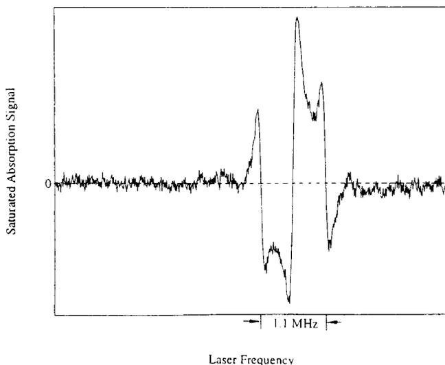
**Fig. 2.** Calcium saturated-absorption signal observed using the system diagrammed in Fig. 1. The lineshape results from the optical-heterodyne detection method using frequency modulation of the laser at 1.1 MHz. This example shows a calcium resonance with a 100 kHz width with a nearly flat background. A good signal-to-noise ratio is achieved even using a 60 kHz detection bandwidth.
