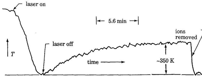
Fig. 6. - The first optical sideband cooling of ions in a Penning trap. The vertical scale is the axial temperature of the  $\text{Mg}^+$  ions as measured from the currents induced in the trap electrodes by the ions' motion. The ions were heated by the laser before the beginning of the data. The laser was turned on with a frequency below the resonance frequency, cooling the ions to below 40 K. After the laser is turned off, the ions thermalize to the ambient temperature of 350 K.
