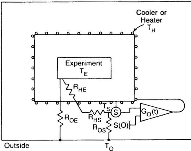
Fig. 1 Schematic representation of an experiment contained within an oven shell. The various temperatures are represented by T's and the thermal impedances by R's.  $T_S(0)$  is the set point of the oven, and S is the thermal sensor.
