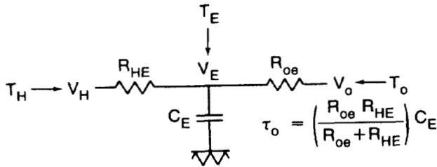
Fig. 6 Electrical analog for the thermal circuit of the heater/cooler, thermal sensor, experiment showing the various couplings.
