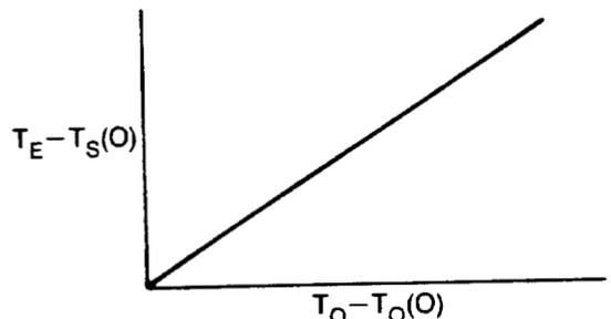
Fig. 4 Steady state temperature error of the experiment,  $T_E$  versus changes in the outside temperature,  $T_0$ , from its nominal value  $T_0(0)$ . The slope of this line yields a good estimate of  $R_{HE}/R_{OE}$ .
