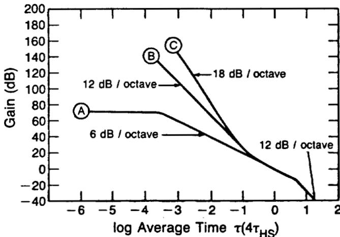
Fig. 2 Oven servo gain  $G_0(\tau)$  in dB versus averaging time (measurement time) in units of  $4\tau_{HS}$  for proportional gain in curve A, for proportional gain plus one integrator with  $\beta=4$  in curve B, and proportional gain plus 2 integrators with  $\beta=4$  in curve c.
