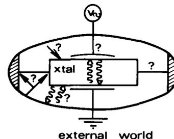
FIGURE 1 Schematic diagram showing the coupling of a crystal resonator to the real world.
