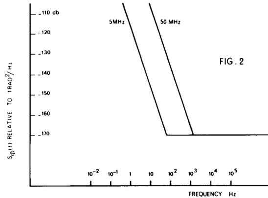
FIGURE 2 Spectral density of phase fluctuations of idealized and 5 MHz and 10 MHz oscillators.
