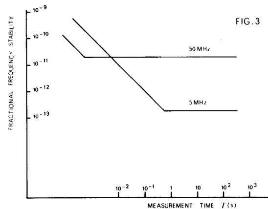
FIGURE 3 Fractional frequency stability,  $\sigma_y(\tau)$ , as a function of measurement time  $\tau$ .
