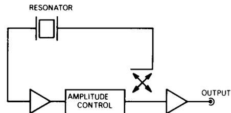
FIGURE 4 Block diagram of a crystal oscillator.
