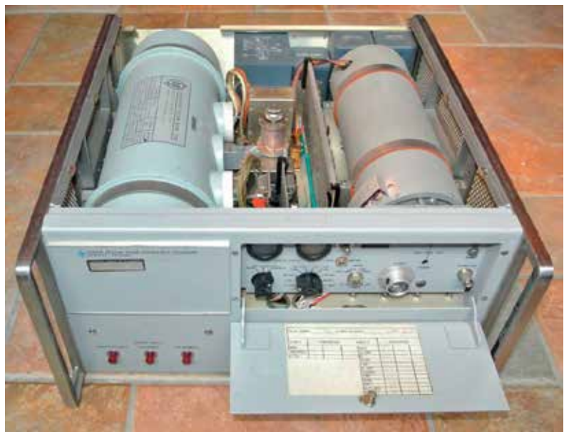
Figure 9: Hewlett-Packard 5060A cesium beam atomic clock with cover removed showing beam tube on left (courtesy of Tom Van Baak, leapsecond.com).
