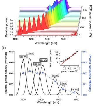
Fig. 2. (Color online) (a) Soliton shift as a function of launch power into the PCF, with each spectrum individually normalized. (b) MIR idler spectra and conversion efficiency relative to pump photons. The total average power is also noted above each spectrum. The absorption feature at  $4.4\,\mu\mathrm{m}$  is due to airpath absorption of  $\mathrm{CO}_2$  before the monochromator. Inset: average idler power as function of pump power at the  $\sim 3.2\,\mu\mathrm{m}$  tuning point.
