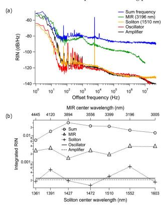
Fig. 3. (Color online) (a) Relative intensity noise (RIN) for the MIR tuning point of  $3.196\,\mu\text{m}$ . Measurement of the MIR RIN is limited to 10 MHz due to photodiode bandwidth. (b) Integrated RIN (10 Hz–10 MHz).
