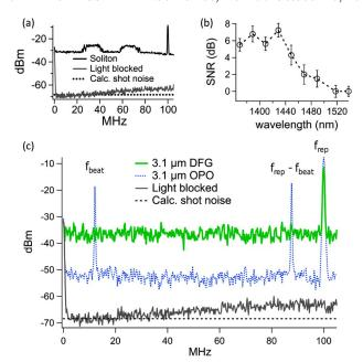
Fig. 4. (Color online) Coherence properties of the system. (a) Free-running beat note between the  $1.36\,\mu\mathrm{m}$  soliton and CW laser with the max-hold function enabled over several seconds of measurement; the spread in beat-note frequency is due to variation in the unlocked repetition rate of the Yb:fiber oscillator. (b) Beat note signal-to-noise ratio across the soliton tuning range. (c) MIR beat notes.
