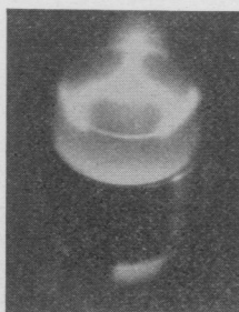
Fig. 15—174 kc, mounting B , height 36.67 mm, dia. 24.715 mm.
